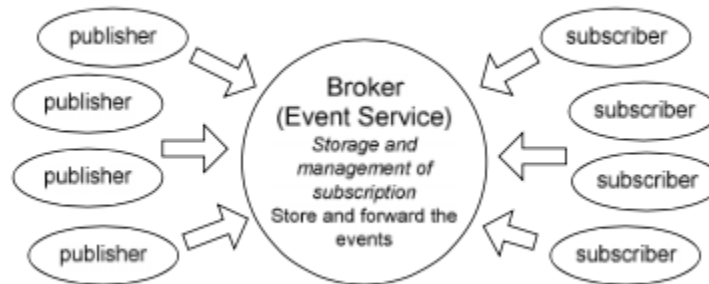
Figure 1. The publish/subscribe system components and basic diagram [11].
